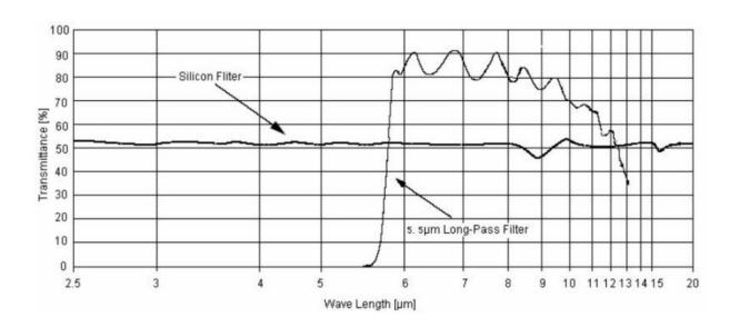
Note: This chart is typical 5um infrared filter, and the curve is the average value of infrared pass rate. This window material is a semiconductor wafer, which is processed by special vacuum coating.
