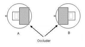
Dual sensor sensitivity balance degree can be got by detecting each cell's sensitivity (single signal output peak) and calculate in following formula:
