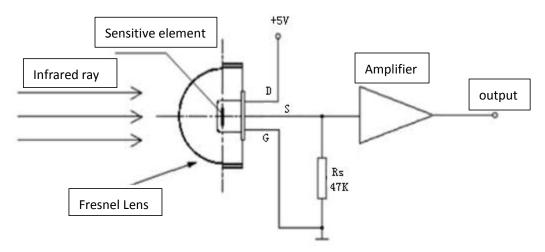
By using different Fresnel lens, the detection range and distance can be determined. According to customer's requirement, it can response to various detection range and distance.
